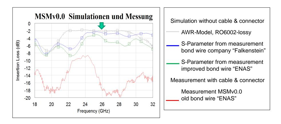
Simulated losses after optimisation of technique for joining parts Without cable and connector: 3...4 dB, cable and connector : 7...8 dB
